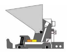
Cleans and evacuates any atmosphere side deposits by circulation of another pressure-free fluid coming from an external source.
