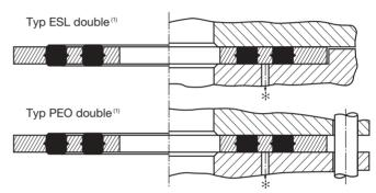
Ensures metal-to-metal contact of joint faces in single or double recess flanges.
